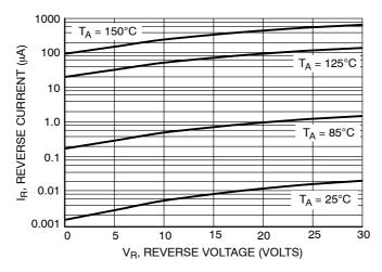
Figure 3. Leakage Current
