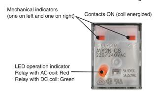
Relay with AC Coil (LED: Red)
