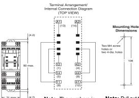
Note: The numbers in parentheses are traditionally used terminal numbers. **Note:** Pull out the hooks to mount the Relay with screws.
