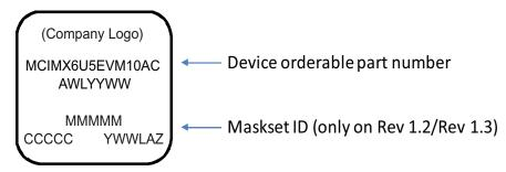
Figure 2. Example Part Marking for Revision 1.2/1.3 Devices
