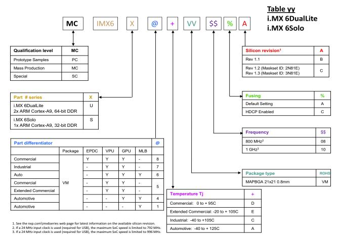
Figure 1. Revision Level to Part Marking Cross-Reference
