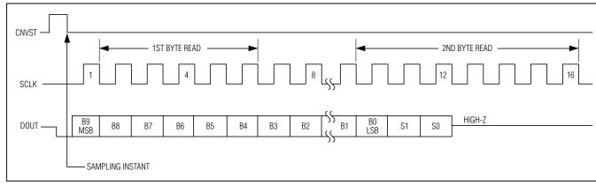
Figure 8c. SPI/MICROWIRE Interface Timing Sequence (CPOL = CPHA = 0)
