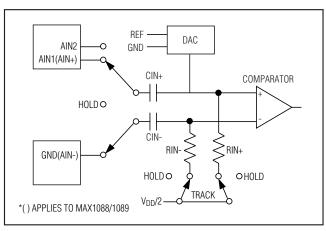
Figure 4. Equivalent Input Circuit
