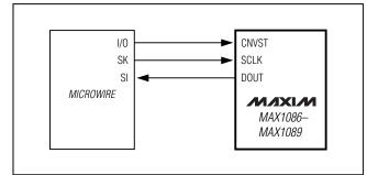
Figure 8b. MICROWIRE Connections
