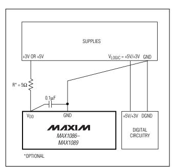
Figure 11. Power-Supply and Grounding Connections
