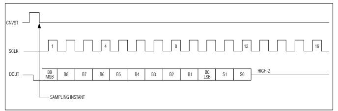
Figure 9b. QSPI Interface Timing Sequence (CPOL = CPHA = 0)
