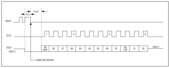
Figure 5b. Single Conversion AIN2 vs. GND (MAX1086/MAX1087), bipolar mode AIN+ vs. AIN- (MAX1088/MAX1089)
