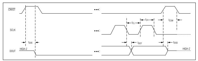
Figure 1. Detailed Serial-Interface Timing Sequence
