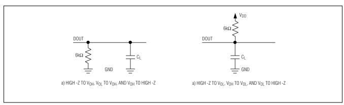
Figure 2. Load Circuits for Enable/Disable Times
