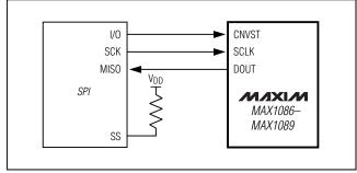
Figure 8a. SPI Connections
