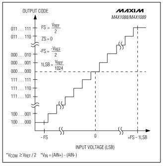
Figure 7. Bipolar Transfer Function
