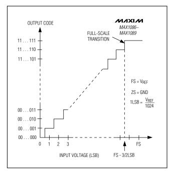
Figure 6. Unipolar Transfer Function
