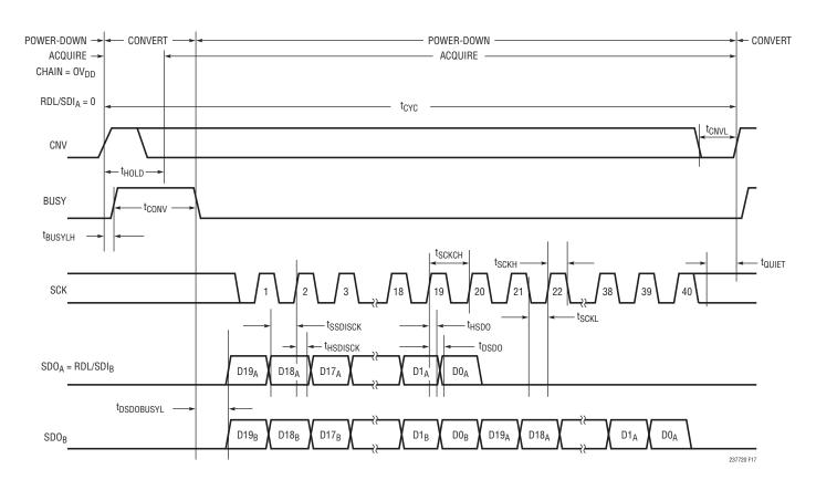
Figure 17. Chain Mode Timing Diagram
