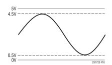
Figure 10. Input Swing of the LTC2377 with Gain Compression Enabled
