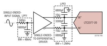
Figure 4. Input Signal Chain
