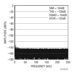
Figure 13. 128k Point FFT Plot with  $f_{IN} = 2kHz$  of the LTC2377-20
