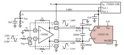
Figure 11a. LTC6362 Configured to Accept a ±3.28V Input Signal While Running from a Single 5V Supply When Digital Gain Compression Is Enabled in the LTC2377-20
