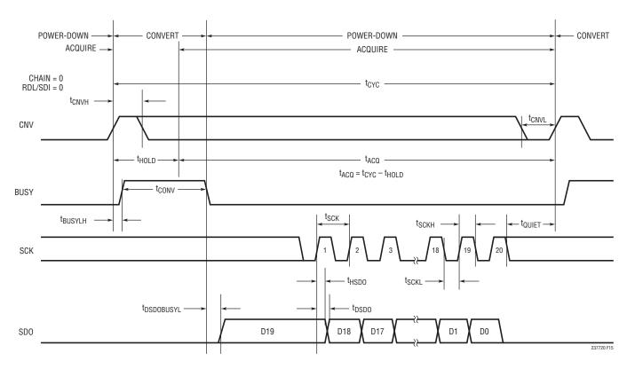
Figure 15. Using a Single LTC2377-20 in Normal Mode
