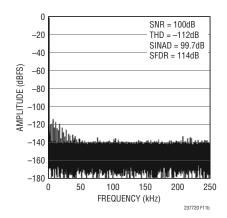
Figure 11b. 64k Point FFT Plot with f<sub>IN</sub> = 2kHz for Circuit Shown in Figure 11a
