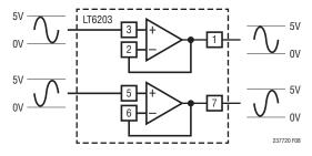
Figure 8. LT6203 Buffering a Fully Differential Signal Source
