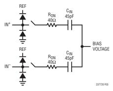
Figure 3. The Equivalent Circuit for the Differential Analog Input of the LTC2377-20
