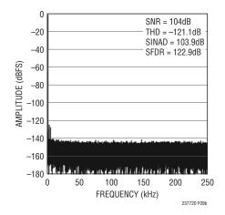
Figure 9b. 128k Point FFT Plot with  $f_{\text{IN}}$  = 2kHz for Circuit Shown in Figure 9a
