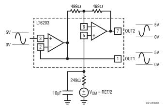
Figure 9a. LT6203 Converting a OV to 5V Single-Ended Signal to a ±5V Differential Input Signal
