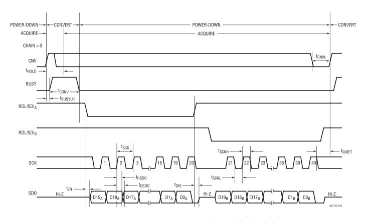
Figure 16. Normal Mode With Multiple Devices Sharing CNV, SCK and SDO
