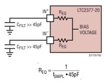
Figure 5. Equivalent Circuit for the Differential Analog Input of the LTC2377-20 at 500ksps.
