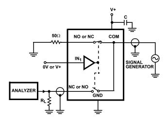
FIGURE 6. CROSSTALK TEST CIRCUIT
