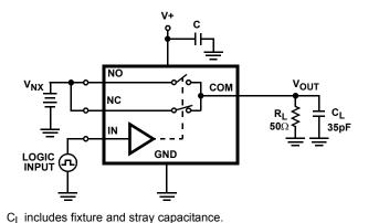
FIGURE 3A. MEASUREMENT POINTS
