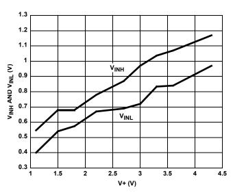
FIGURE 17. DIGITAL SWITCHING POINT vs SUPPLY VOLTAGE
