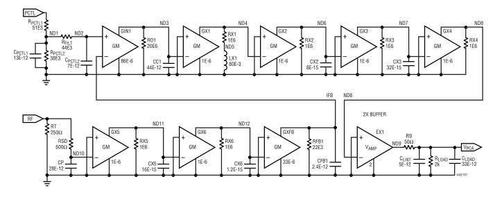
Figure 7. LTC4402 Low Frequency AC Model
