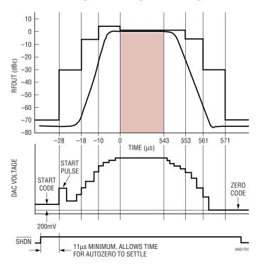
Figure 1. LTC4402 Ramp Timing
