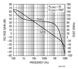
Figure 5. SPICE Model Open Loop Gain and Phase Characteristics from RF to V<sub>PCA</sub>, PCTL <80mV
