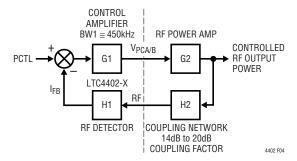
Figure 4. Closed Loop Block Diagram
