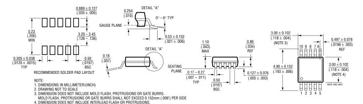
INTERLEAD FLASH OR PROTRUSIONS SHALL NOT EXCEED 0.152mm (.006") PER SIDE 5. LEAD COPLANARITY (BOTTOM OF LEADS AFTER FORMING) SHALL BE 0.102mm (.004") MAX
