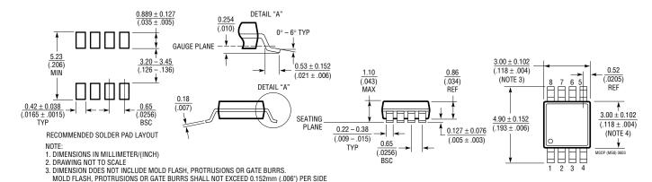
4. DIMENSION DOES NOT INCLUDE INTERLEAD FLASH OR PROTRUSIONS. INTERLEAD FLASH OR PROTRUSIONS SHALL NOT EXCEED 0.152mm (.006") PER SIDE
