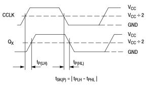
Figure 10. Output Pulse Skew (t<sub>SK(P)</sub>) Test Reference
