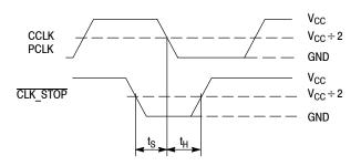
Figure 14. Setup and Hold Time (t<sub>S</sub>, t<sub>H</sub>) Test Reference
