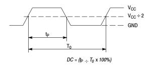
The time from the output controlled edge to the non-controlled edge, divided by the time between output controlled edges, expressed as a percentage
