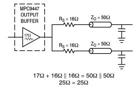
Figure 6. Optimized Dual Line Termination
