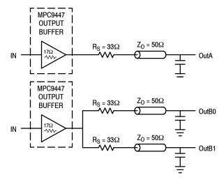
Figure 4. Single versus Dual Transmission Lines
