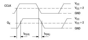
Figure 8. Propagation Delay (t<sub>PD</sub>) Test Reference
