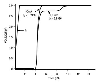
Figure 5. Single versus Dual Line Termination Waveforms
