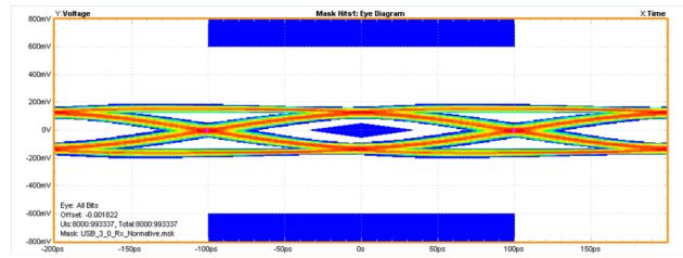
Figure 4. 5 Gbps Eye Diagram with Eye Mask
