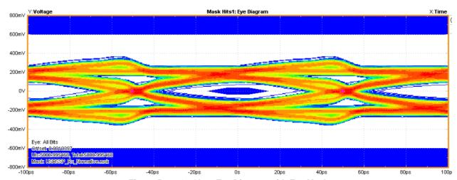
Figure 5. 10 Gbps Eye Diagram with Eye Mask
