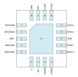
Figure 3. Pin Assignment (Top Through View)
