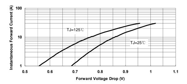
Fig.3-Typical Instantaneous Forward Voltage Characteristics
