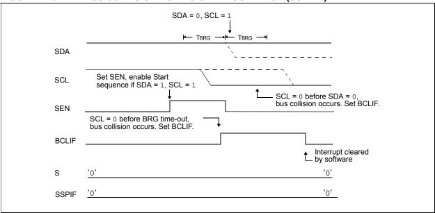
FIGURE 21-35: BRG RESET DUE TO SDA ARBITRATION DURING START CONDITION
