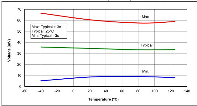
FIGURE 26-53: BROWN-OUT RESET VOLTAGE, BORV = 0
