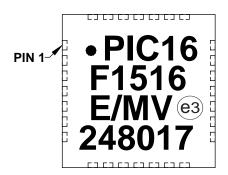
28-Lead QFN (6x6x0.9 mm)
