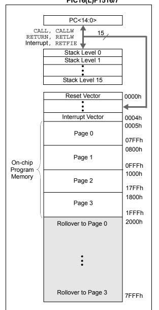
FIGURE 3-2: PROGRAM MEMORY MAP AND STACK FOR PIC16(L)F1518/9
