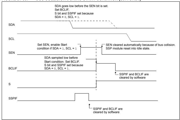
FIGURE 21-34: BUS COLLISION DURING START CONDITION (SCL = 0)
