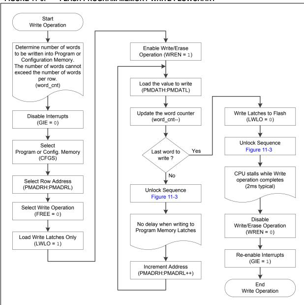
FIGURE 11-6: FLASH PROGRAM MEMORY WRITE FLOWCHART
