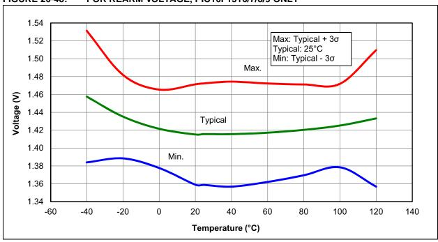
FIGURE 26-49: BROWN-OUT RESET VOLTAGE, BORV = 1, PIC16LF1516/7/8/9 ONLY
