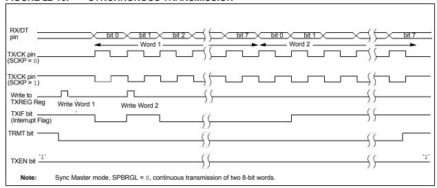
FIGURE 22-11: SYNCHRONOUS TRANSMISSION (THROUGH TXEN)
