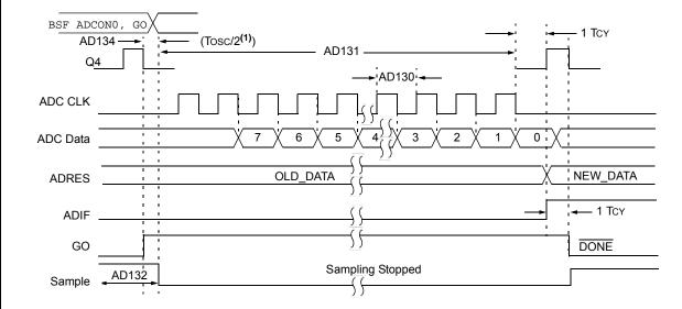
Note 1: If the ADC clock source is selected as FRC oscillator, a time of TCY is added before the ADC clock starts. This allows the SLEEP instruction to be executed.
