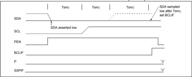
FIGURE 21-39: BUS COLLISION DURING A STOP CONDITION (CASE 2)
