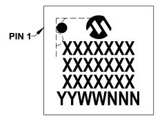
44-Lead TQFP (10x10x1 mm)
