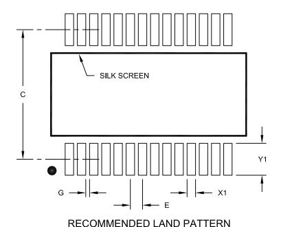
**MILLIMETERS** Units **Dimension Limits** MIN MOM MAX Contact Pitch 0.65 BSC Ε С Contact Pad Spacing 7.20 X1 0.45 Contact Pad Width (X28) Contact Pad Length (X28) Y1 1.75 0.20 Distance Between Pads G
