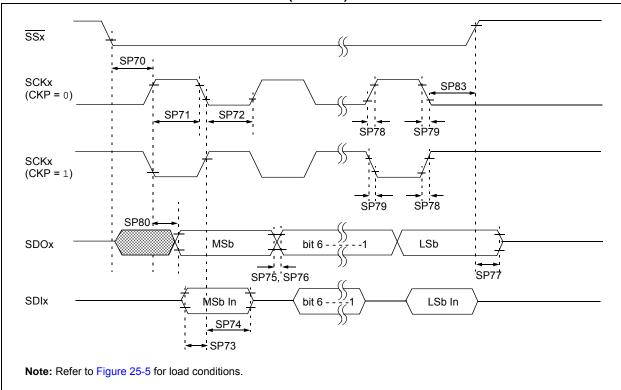
FIGURE 25-19: SPI SLAVE MODE TIMING (CKE = 1)
