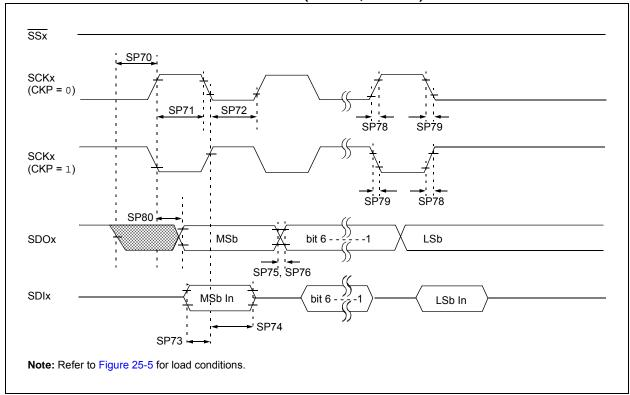
FIGURE 25-17: SPI MASTER MODE TIMING (CKE = 1, SMP = 1)
