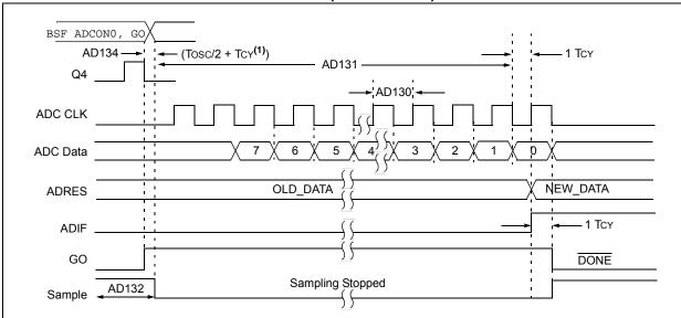
Note 1: If the ADC clock source is selected as FRC oscillator, a time of Tcy is added before the ADC clock starts. This allows the SLEEP instruction to be executed.
