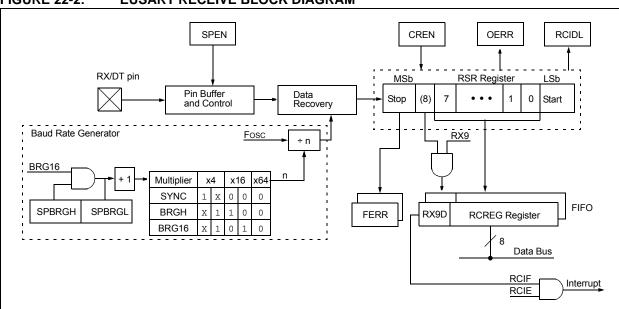
FIGURE 22-2: EUSART RECEIVE BLOCK DIAGRAM
