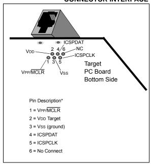
Another connector often found in use with the PICkit™ programmers is a standard 6-pin header with 0.1 inch spacing. Refer to Figure 23-2.
