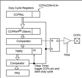
Note 1: The 8-bit timer TMR2 register is concatenated with the 2-bit internal system clock (Fosc), or two bits of the prescaler, to create the 10-bit time base
