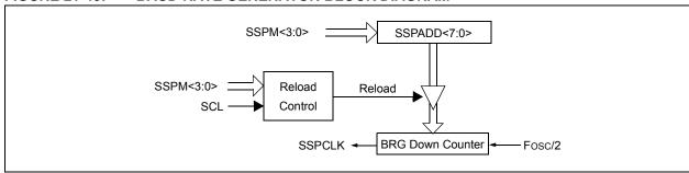
**lote:** Values of 0x00, 0x01 and 0x02 are not valid for SSPADD when used as a Baud Rate Generator for I<sup>2</sup>C. This is an implementation limitation.
