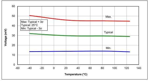
FIGURE 26-51: BROWN-OUT RESET VOLTAGE, BORV = 1, PIC16F1516/7/8/9 ONLY
