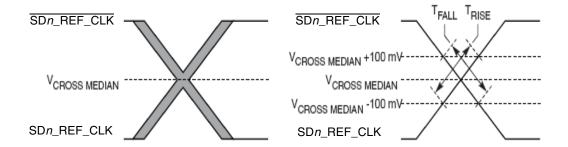
Figure 48. Single-Ended Measurement Points for Rise and Fall Time Matching
