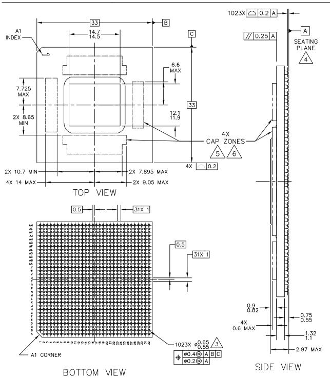
Figure 57. MPC8641D High-Head FC-CBGA Dimensions
