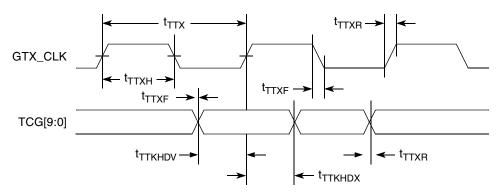
Figure 16. TBI Transmit AC Timing Diagram
