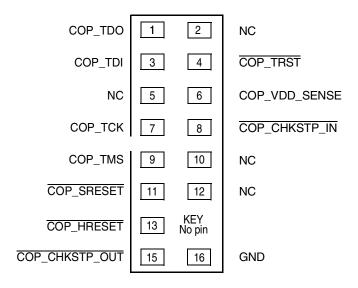
Figure 67. COP Connector Physical Pinout
