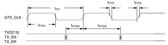
Figure 8. FIFO Transmit AC Timing Diagram
