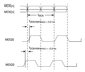
Figure 5. Timing Diagram for tDDKHMH
