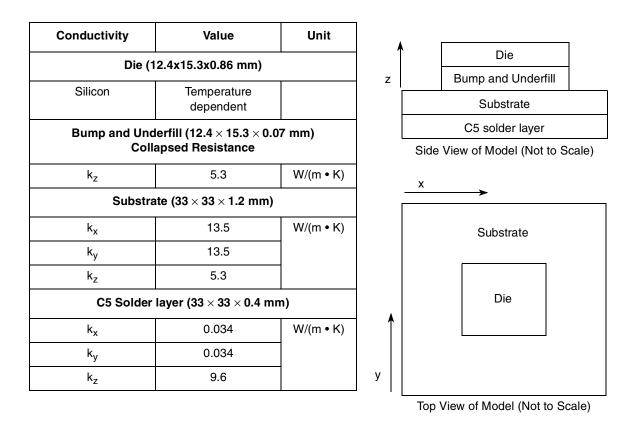
Figure 62. Recommended Thermal Model of MPC8641
