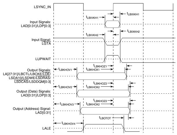
Figure 26. Local Bus Signals (PLL Enabled)
