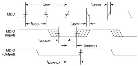
Figure 24. MII Management Interface Timing Diagram
