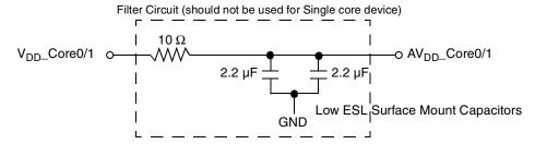
**Note:** For single core device the filter circuit (in the dashed box) should be removed and  $AV_{DD}$ \_Core1 should be tied to ground with a weak (2-10 k $\Omega$ ) pull-down resistor.
