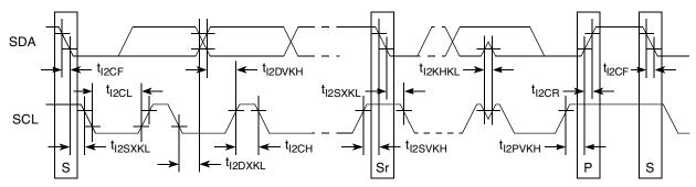
Figure 37. I<sup>2</sup>C Bus AC Timing Diagram
