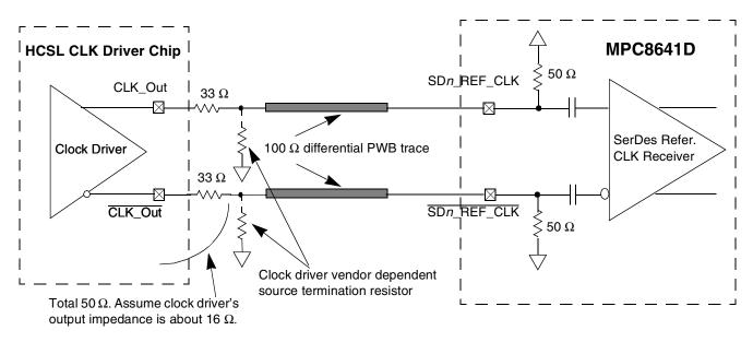
Figure 43. DC-Coupled Differential Connection with HCSL Clock Driver (Reference Only)
