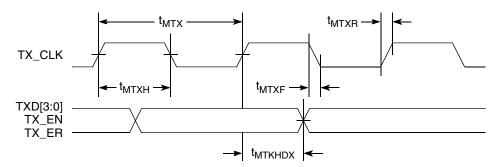
Figure 13. MII Transmit AC Timing Diagram
