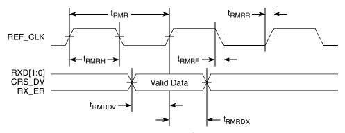
Figure 22. RMII Receive AC Timing Diagram
