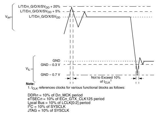
Figure 2. Overshoot/Undershoot Voltage for Dn\_M/O/L/TV<sub>IN</sub>
