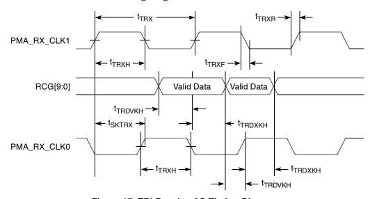
Figure 17. TBI Receive AC Timing Diagram
