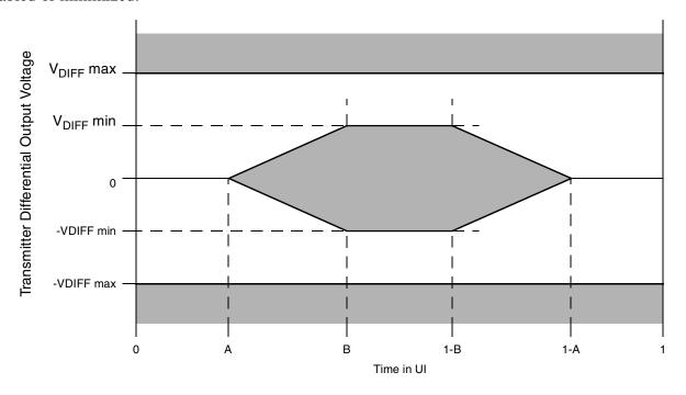
Figure 54. Transmitter Output Compliance Mask
