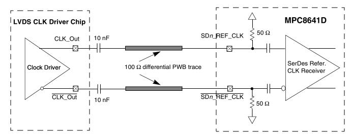
Figure 44. AC-Coupled Differential Connection with LVDS Clock Driver (Reference Only)
