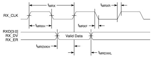
Figure 15. MII Receive AC Timing Diagram
