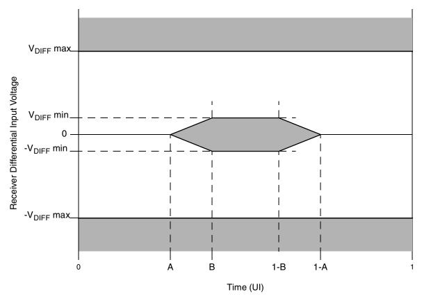
Figure 56. Receiver Input Compliance Mask
