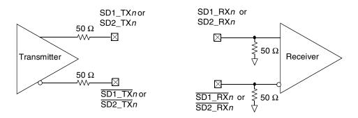
Figure 49. SerDes Transmitter and Receiver Reference Circuits
