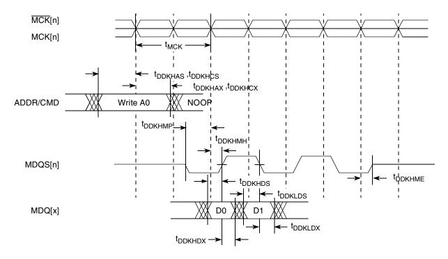
Figure 6. DDR SDRAM Output Timing Diagram
