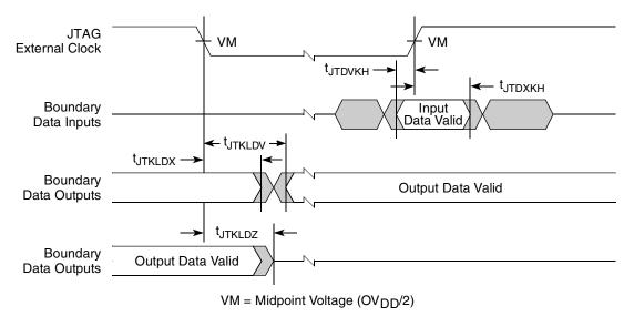
Figure 35. Boundary-Scan Timing Diagram
