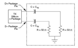
Figure 52. Compliance Test/Measurement Load
