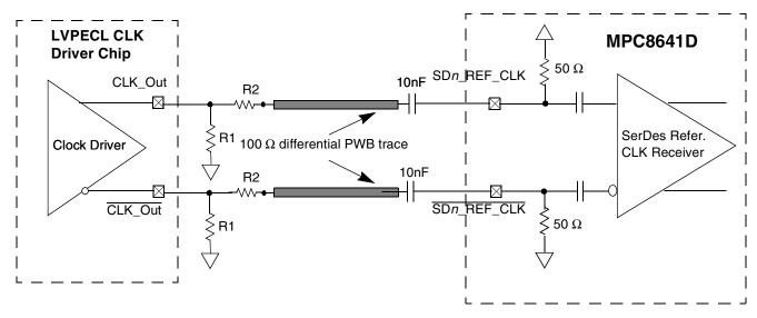
Figure 45. AC-Coupled Differential Connection with LVPECL Clock Driver (Reference Only)
