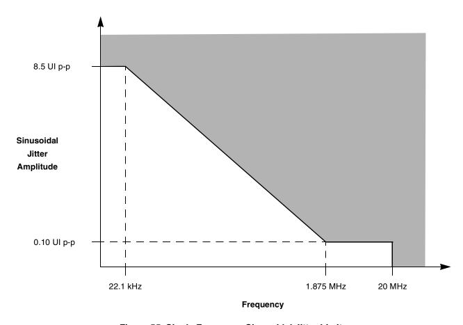
Figure 55. Single Frequency Sinusoidal Jitter Limits
