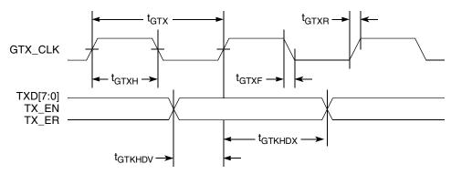
Figure 10. GMII Transmit AC Timing Diagram
