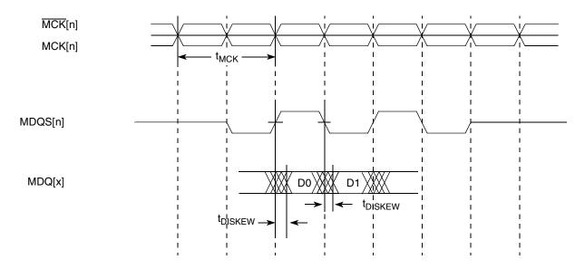
Figure 4. DDR Input Timing Diagram for tDISKEW
