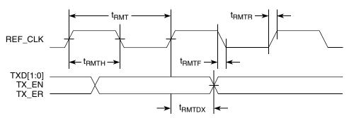
Figure 20. RMII Transmit AC Timing Diagram
