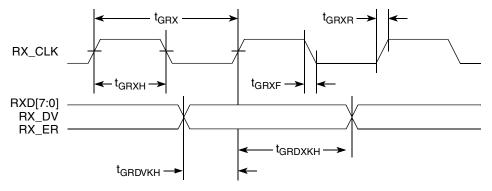
Figure 12. GMII Receive AC Timing Diagram
