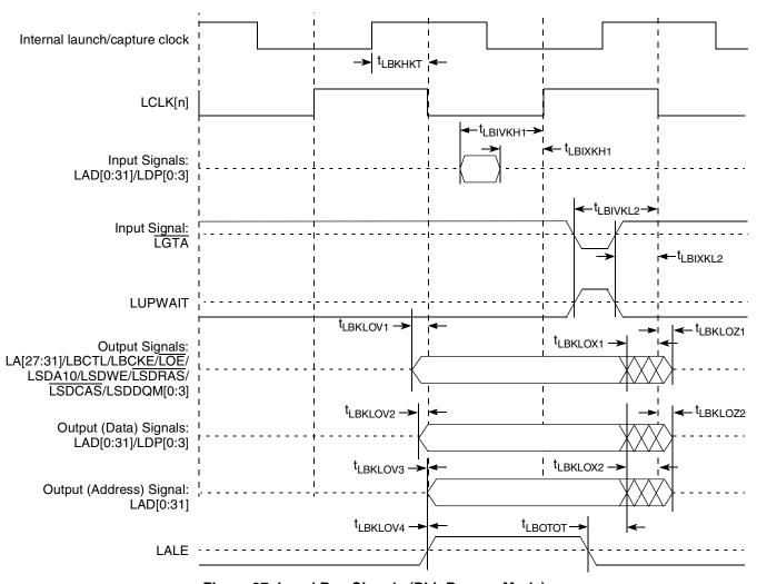
Figure 27. Local Bus Signals (PLL Bypass Mode)
