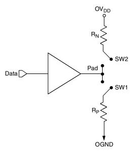
Figure 66. Driver Impedance Measurement
