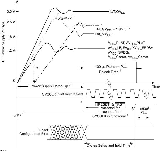
Figure 3 illustrates the Power Up sequence as described above.
