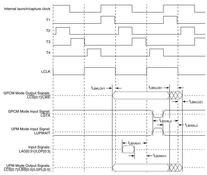
Figure 31. Local Bus Signals, GPCM/UPM Signals for LCRR[CLKDIV] = 4 or 8 (clock ratio of 8 or 16) (PLL Bypass Mode)
