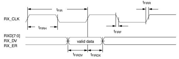
Figure 9. FIFO Receive AC Timing Diagram
