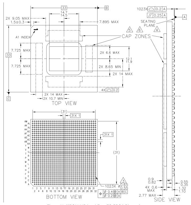
Figure 58. MPC8641D Lead-Free FC-CBGA Dimensions
