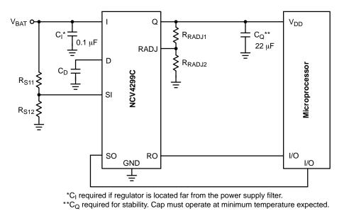
Figure 35. Test and Application Circuit Showing all Compensation and Sense Elements for 8 Pin Package Part
