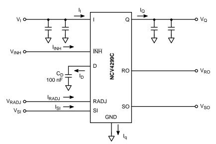
Figure 3. Measurement Circuit
