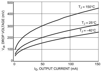
Figure 7. Drop Voltage vs. Output Current
