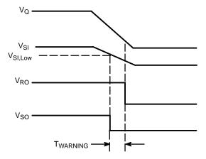
Figure 37. SO Warning Timing Waveform
