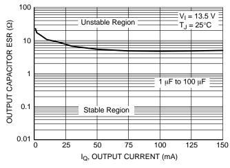
Figure 18. Output Stability vs. Output Capacitor ESR
