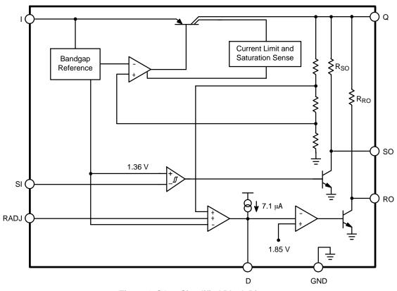
Figure 1. SO–8 Simplified Block Diagram
