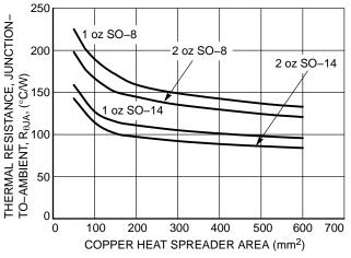
Figure 39. Thermal Resistance  $R_{\theta JA}$  vs. Copper Area
