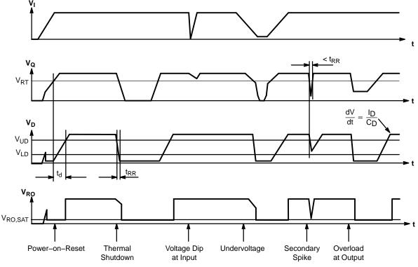
Figure 36. Reset Timing Diagram
