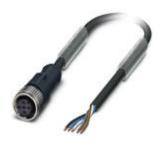
Sensor/Actuator cable, 5-position, PUR halogen-free, black-gray RAL 7021, free cable end, on Socket straight M12, B-coded, Cable length: 6 m
