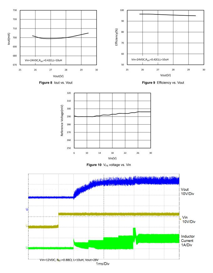
Figure 11 Soft-start waveform
