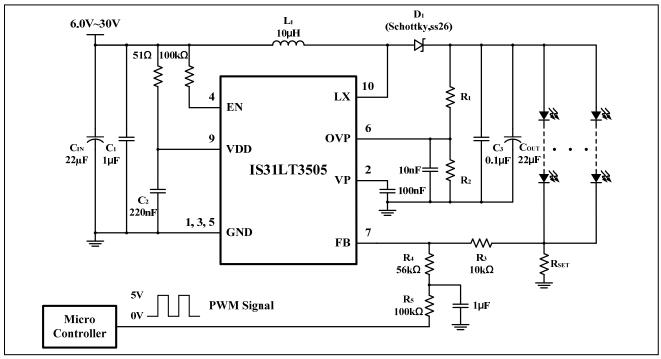
Figure 15 Application Circuit (Constant Current to Drive White LEDs With PWM Dimming)
