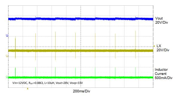
Figure 13 OVP waveform
