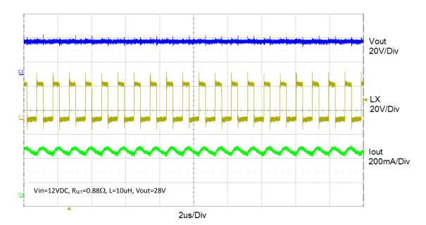
Figure 12 Operation waveform
