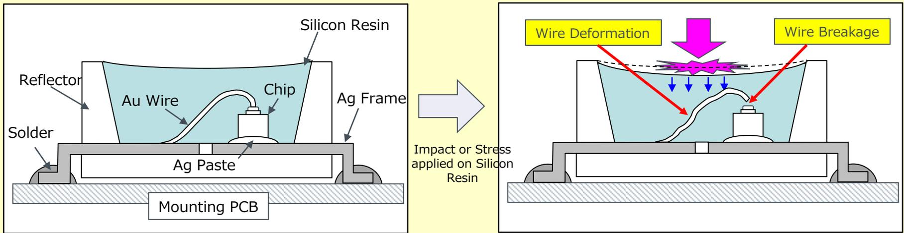
When it is mounting, please have the adsorption collet touching with reflector. After it is mounted, please be care to handle with the part of sealing.
