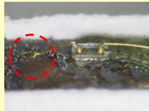
The Ag pattern in the LED case is corroded and color changed into black → wire delamination
