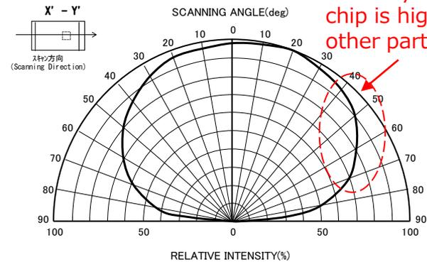
Luminous intensity near the chip is higher than other parts
