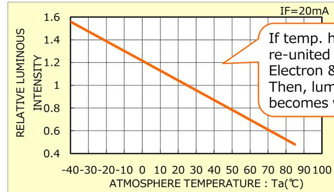
If temp. heating-up, re-united ratio of Electron & hole drops. Then, luminous intensity becomes weak.
