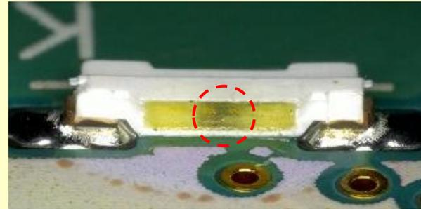
The Ag of frame is corroded and its color changed into black
