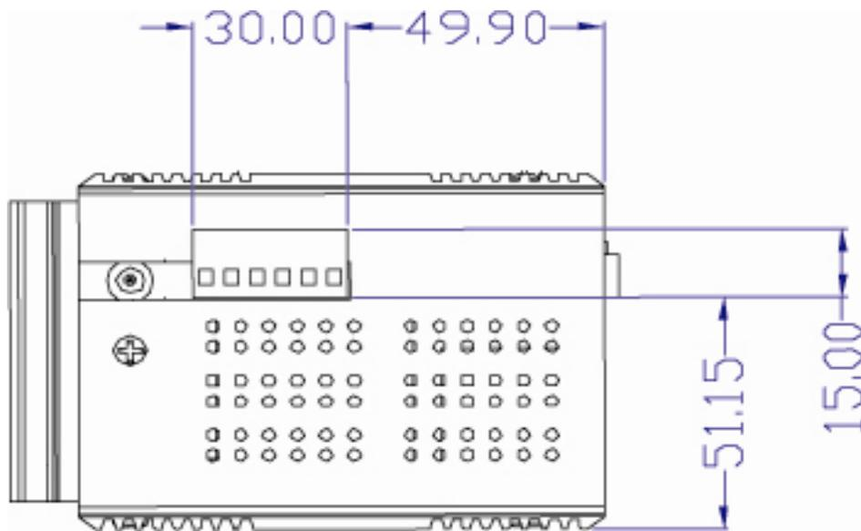
Figure 2.4: Top View of EKI-7659CPI
