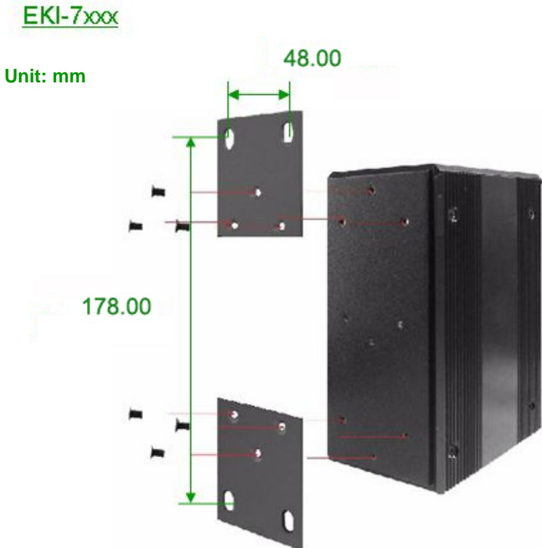
Figure 2.5: Combine the Metal Mounting Kit
