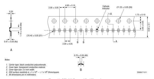
Figure 11. SOD-882 Tape and Reel Dimensions
