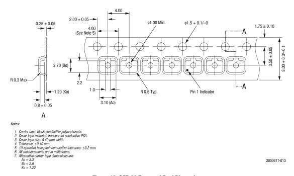
Figure 13. SOT-23 Tape and Reel Dimensions
