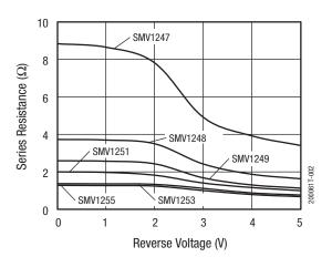
Figure 2. Series Resistance vs Reverse Voltage @ 500 MHz
