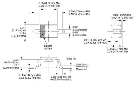
Dimensions are in inches (millimeters shown in parentheses)
