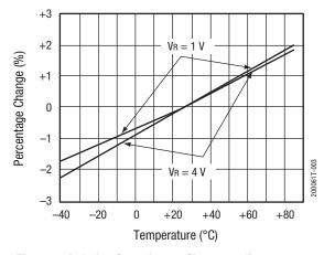
Figure 3. Relative Capacitance Change vs Temperature
