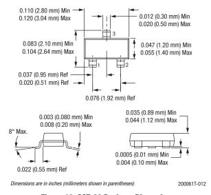
Figure 12. SOT-23 Package Dimensions
