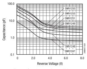
Figure 1. Capacitance vs Reverse Voltage
