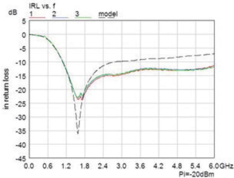
The experimental output return loss (ORL) is better than  $-10$  dB over 1.4–2.7 GHz or 67 percent fractional bandwidth. Therefore, it is the output match that limits the design's usable bandwidth. The ORL variation between the three samples is less than 0.5 dB. The experimental ORL is lowest at 2.1 GHz, but the model predicts a null at 2.6 GHz.
