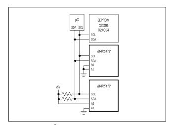
Figure 5. Typical I<sup>2</sup>C Application Circuit
