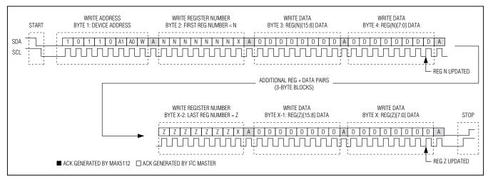
Figure 3. I<sup>2</sup>C Multiple Register Write Sequence
