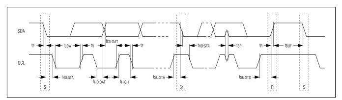
Figure 1. I<sup>2</sup>C Timing Diagram
