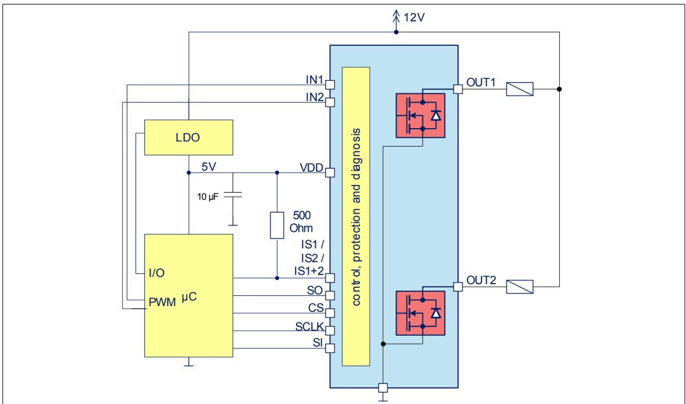
Figure 24 Application Circuit using SPI and Current Sense Output
