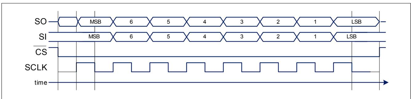
Figure 19 Serial Peripheral Interface
