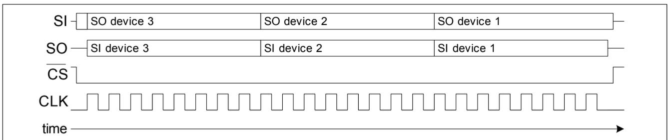
**Figure 21** Data Transfer in Daisy Chain Configuration
