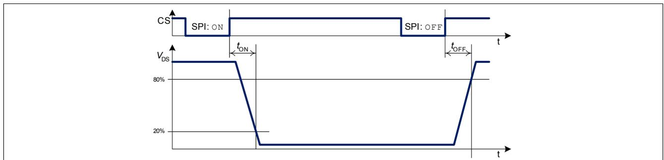
Figure 6 Switching a Resistive Load
