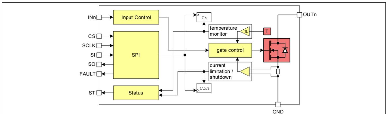
Figure 8 Protection Functions
