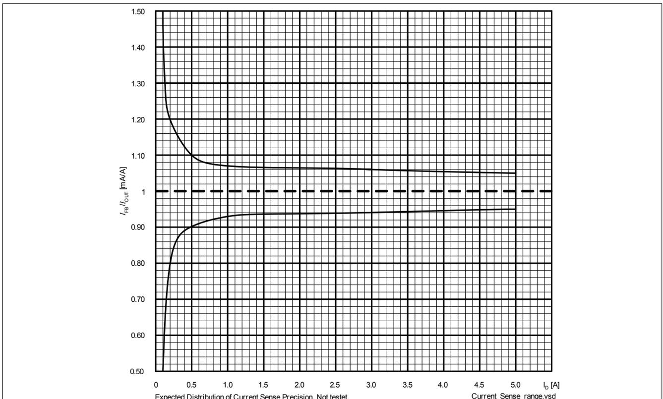
Figure 18 Current Sense Precision - range of expected distribution.
