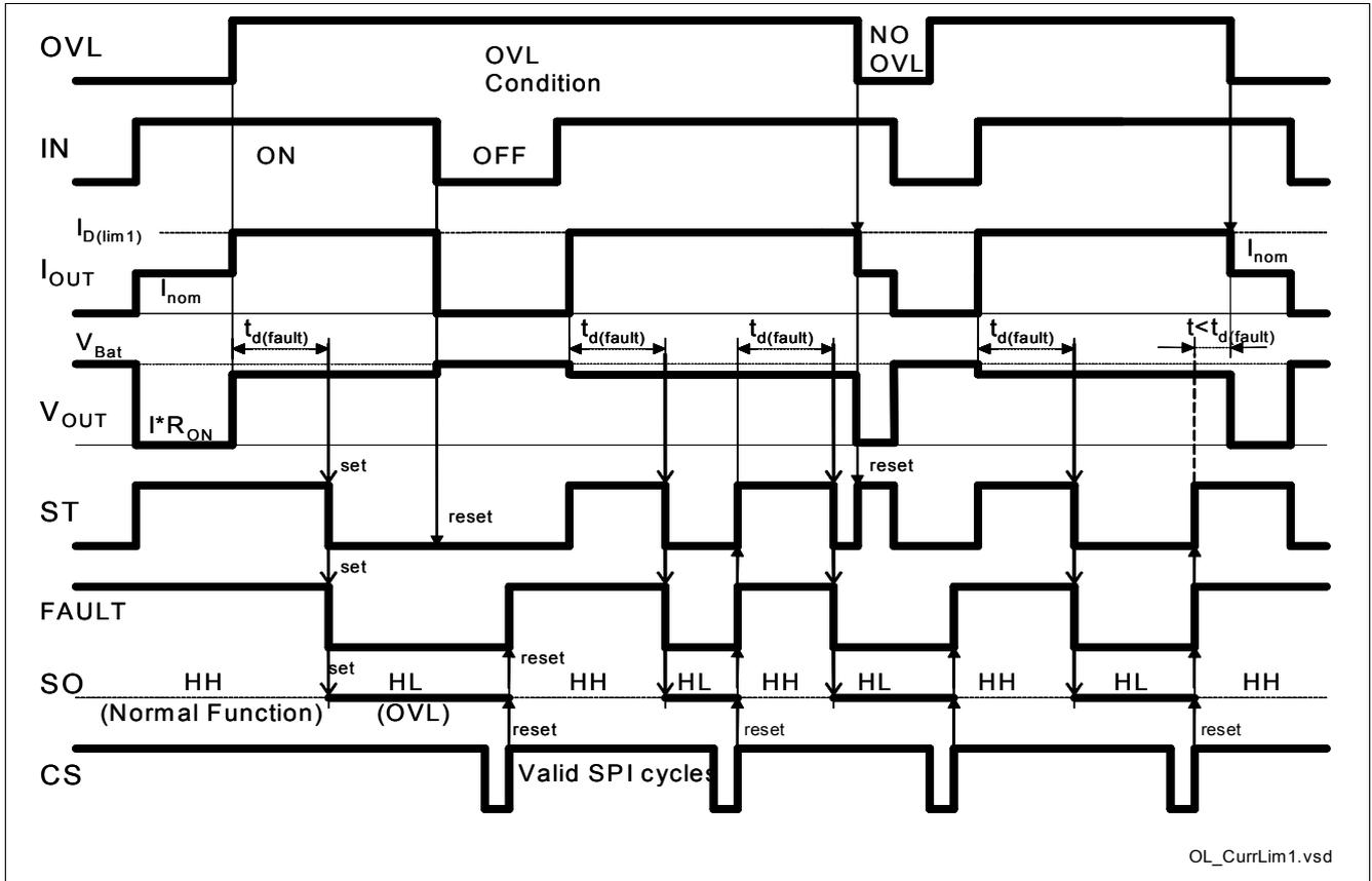
Figure 9 Over Load Behavior - Current Limitation (current limit 1)
