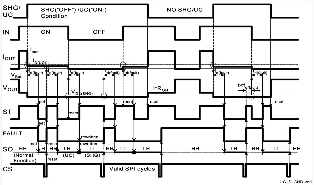
Figure 16 Diagnostic at "Short to GND/Under Current" Condition
