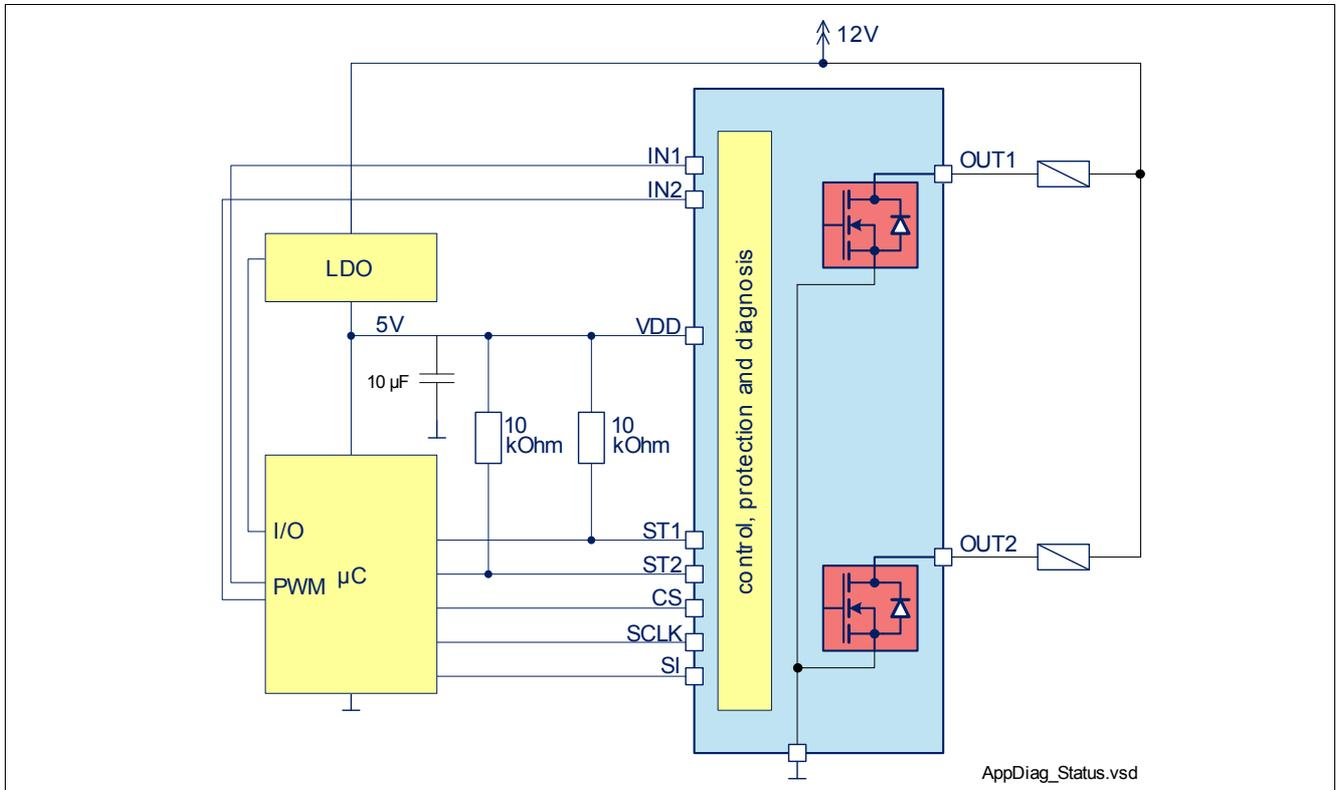
Figure 23 Application Circuit using Status Outputs only
