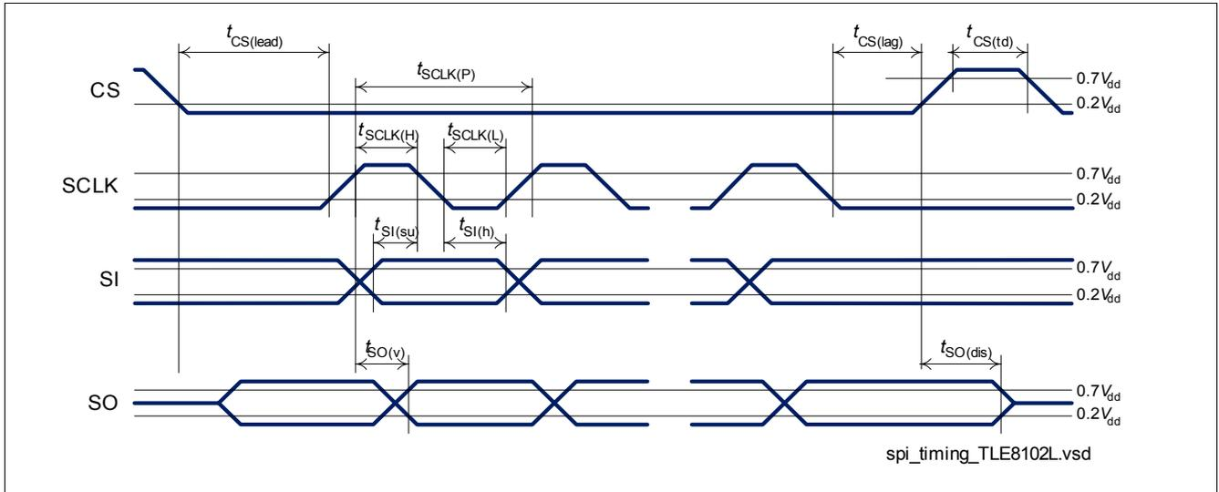
Figure 22 Serial Interface Timing Diagram
