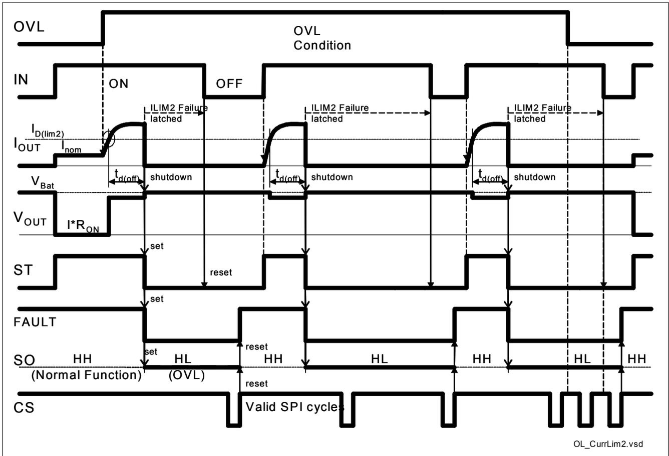
Figure 10 Over Load Behavior - Latched Shutdown (current limit 2)
