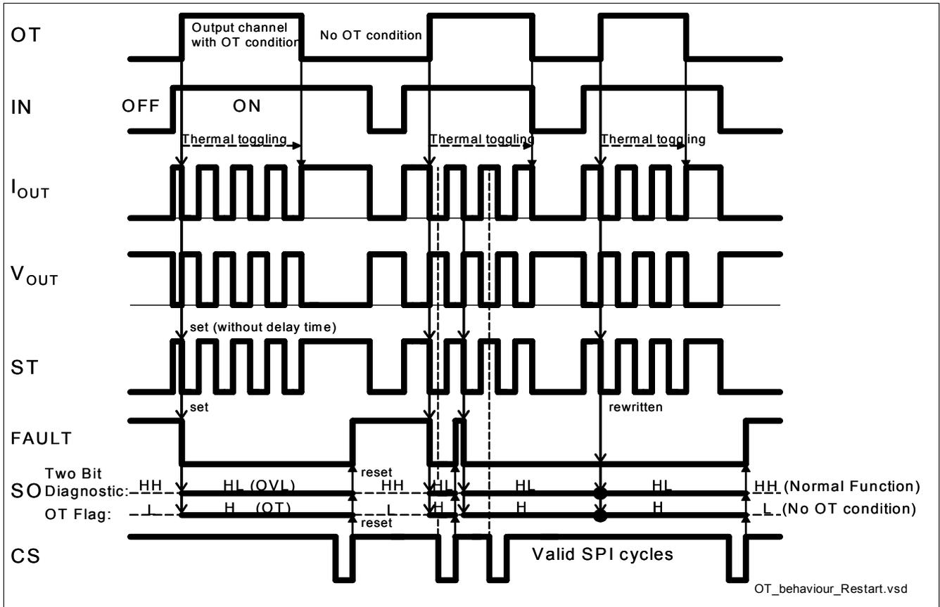
Figure 11 Over Temperature Behavior - Automatic Autorestart
