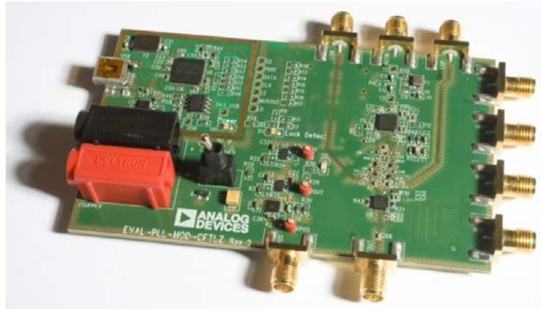
Figure 2. Evaluation Board for CN-0285 Direct Conversion Transmitter
