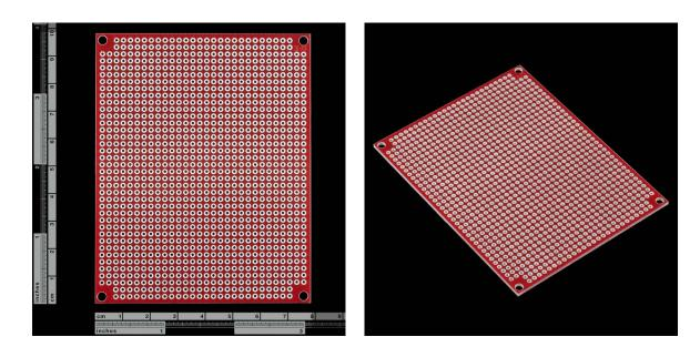
**Description:** An empty canvas for electrical enthusiasts! Designed to fit the SFE project enclosures this project board gives you 8x10cm (3.15x3.94") of building space for through-hole components with 2.54mm (100mil) spaced holes. This is not your normal perf board! This board is much higher quality with plated-through holes and annular rings that will not lift off the PCB under normal soldering conditions.
