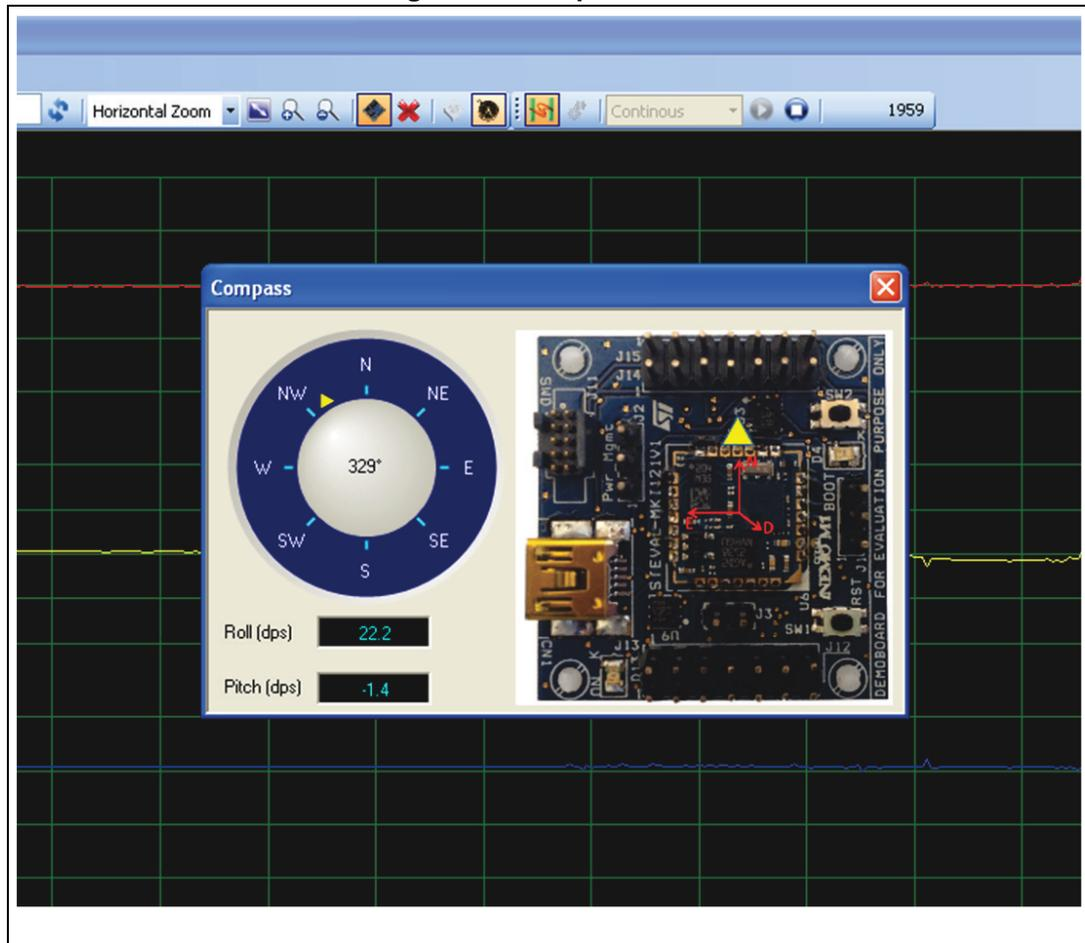
The heading of the board is indicated by the yellow arrow according to the NED system as shown in *Figure 21*. The “Compass” window also shows information on roll and pitch values.
