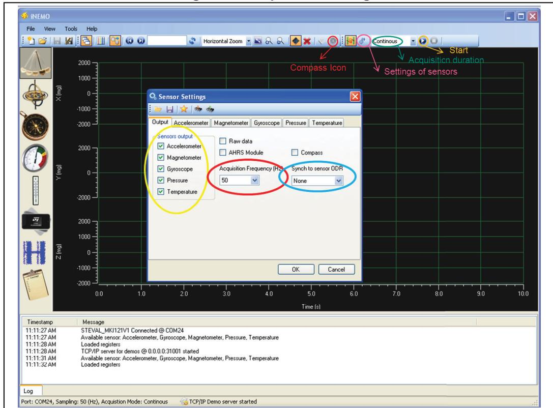
For each sensor it is possible to set parameters like offset, scale factor, output data rate, full scale, as well as other ones related to selecting sensors. The output data rate can be synchronized with the sampling frequency of one sensor selected from the “Sync to sensor ODR” drop-down menu.
