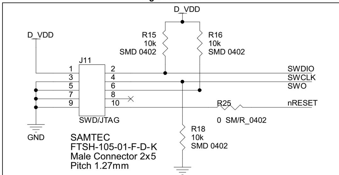
Figure 28. Pinout connectors
