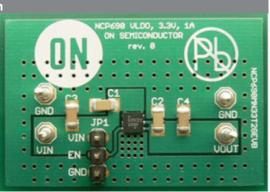
Output Discharge, Current Limit and Thermal Shutdown Protection. Finally the Surface Mount DFN3x3 package with Expose Pad allows saving PCB space and effectively dissipating heat through the PCB copper area. This demonstration board operates from a dc input voltage VIN < 6V and produces fixed output voltage given by the NCP690 internal voltage divider.
