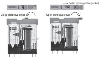
Keep the protective cover open when using the latching lever. Move until the latching lever clicks to the ON position (ON state). After use latching lever, in order to prevent malfunction, return the switch to contact normal position (OFF state), and make sure the protective cover is firmly closed.
