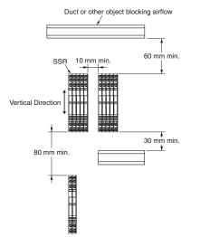
\* When five or more are installed, install with 10 mm space between each.
