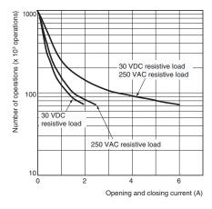
Switching capacity of DC resistive load
