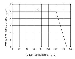
Figure 5. Forward Current Derating Curve
