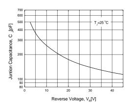
Figure 3. Typical Junction Capacitance (per diode)
