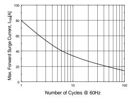
Figure 6. Non-Repetitive Surge Current (per diode)
