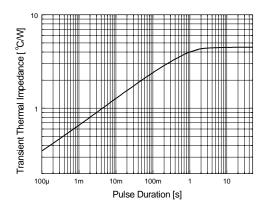
Figure 4. Thermal Impedance Characteristics (per diode)
