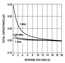
Figure 1. RF Capacitance vs. Reverse Bias.
