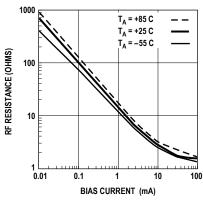
Figure 2. Typical RF Resistance vs. Forward Bias Current.
