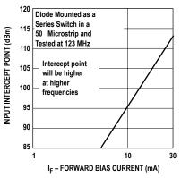
Figure 3. 2nd Harmonic Input Intercept Point vs. Forward Bias Current for Switch Diodes.
