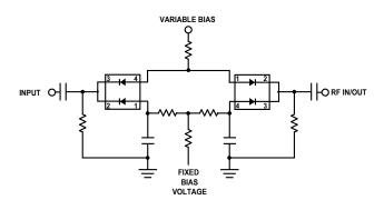
Figure 9. Four Diode  $\boldsymbol{\pi}$  Attenuator. See AN1048 for details.
