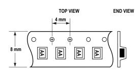
Note: "AA" represents package marking code. Package marking is right side up with carrier tape perforations at top. Conforms to Electronic Industries R5-481, "Taping of Surface Mounted Components for Automated Placement." Standard quantity is 3,000 devices per reel.
