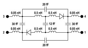
Anti-parallel diode package (HMPP-3862)
