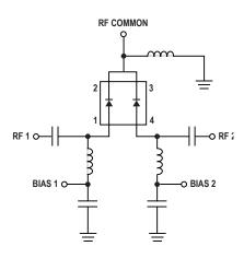
Figure 6. Simple SPDT Switch Using Only Positive Bias.
