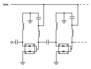
Figure 10. High Isolation SPST Switch (Repeat Cells as Required).
