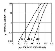
Figure 5. Forward Current vs. Forward Voltage.
