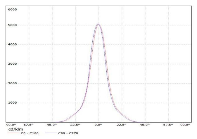
Luminaire: LEDiL CN13107\_LENA-S-DL\_(Soleriq\_E30) Eff. 79% Lamps: 1 x Osram Soleriq E30 (1240lm@250mA)
