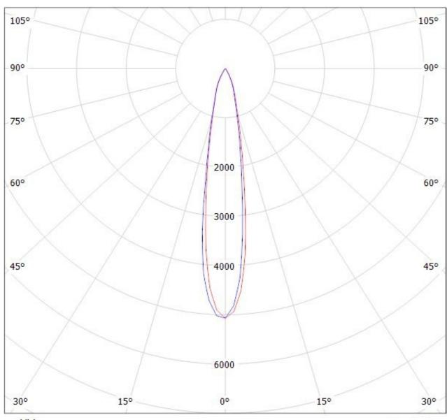
cd/klm C0 - C180 - C90 - C270 NOTE: The typical divergence will be changed by different color, chip size and chip position tolerance. The typical total divergence is the full angle measured where the luminous intensity is half of the peak value.
