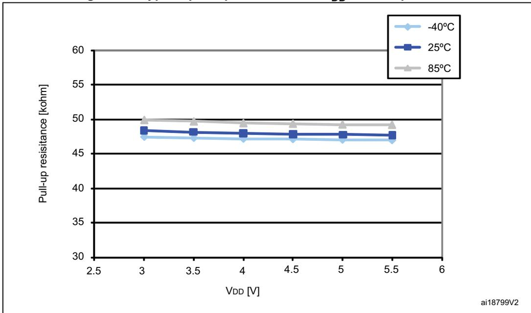
Figure 18. Typical pull-up current vs  $V_{DD}$  @ 3 temperatures
