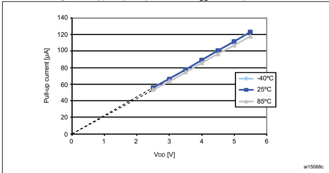
1. The pull-up is a pure resistor (slope goes through 0).
