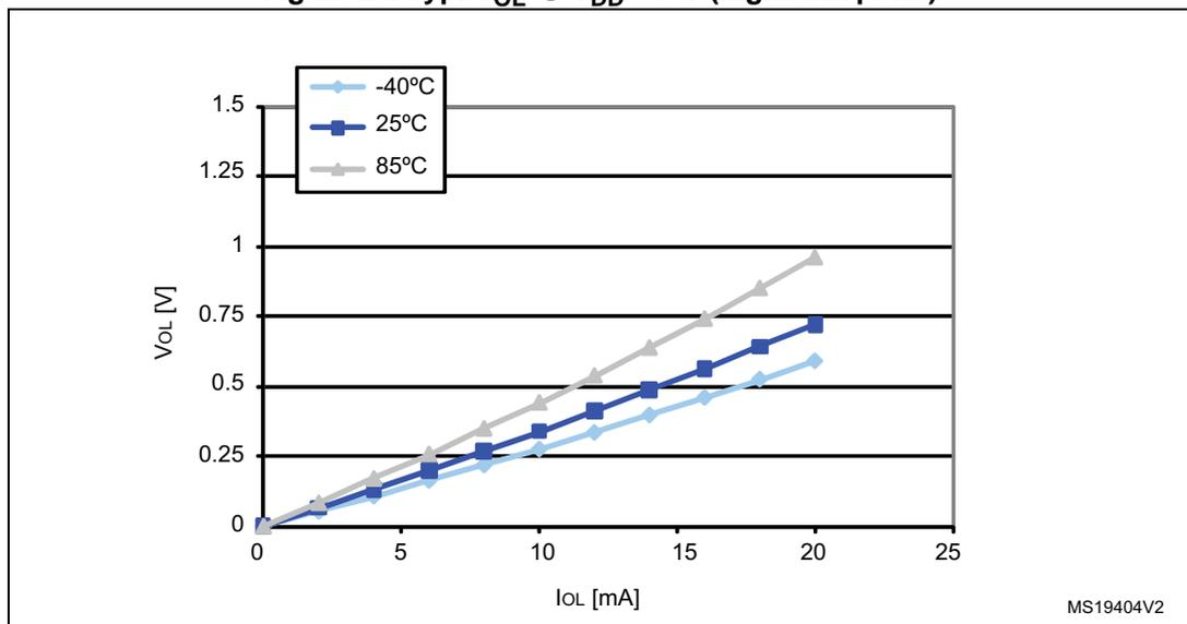
Figure 24. Typ.  $V_{OL}$  @  $V_{DD} = 3.3$  V (high sink ports)
