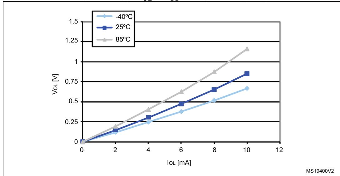
Figure 20. Typ.  $V_{OL}$  @  $V_{DD} = 3.3\text{ V}$  (standard ports)
