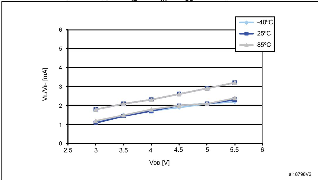
Figure 17. Typical pull-up resistance vs  $V_{DD}$  @ 3 temperatures
