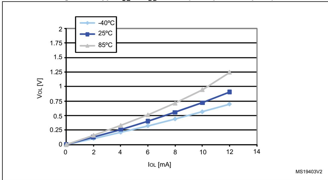
Figure 23. Typ.  $V_{OL}$  @  $V_{DD} = 5$  V (high sink ports)
