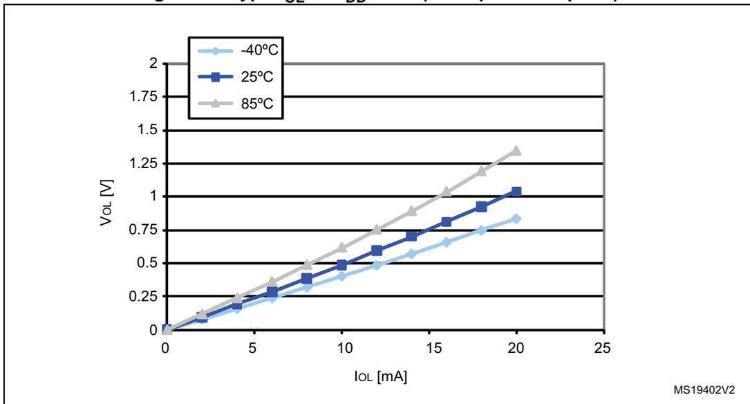
Figure 22. Typ.  $V_{OL}$  @  $V_{DD} = 3.3$  V (true open drain ports)
