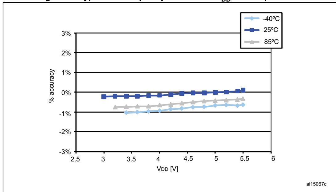
**Low speed internal RC oscillator (LSI)**
