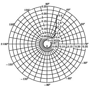
$\begin{array}{l} S_{22e} \\ V_{CE} = 10V \\ I_{C} = 5 mA \\ T_{a} = 25 ^{\circ}C \\ (UNIT:\Omega) \end{array}$
