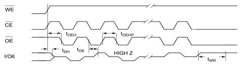
Notes: 1. Toggling either  $\overline{OE}$  or  $\overline{CE}$  or both  $\overline{OE}$  and  $\overline{CE}$  will operate toggle bit. The t<sub>OEHP</sub> specification must be met by the toggling input(s)
