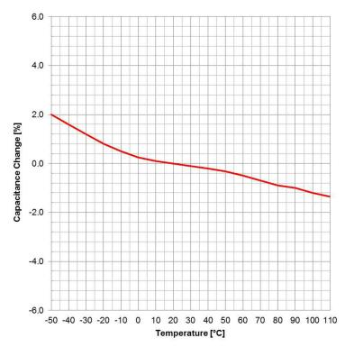
Test Equipment: E4991A or equivalent
