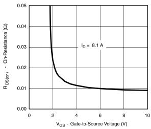
On-Resistance vs. Gate-to-Source Voltage
