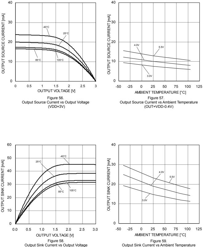
Output Sink Current vs Ambient Temperature (OUT=VSS+0.4V)
