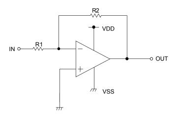
Figure 76. Inverting amplifier circuit
