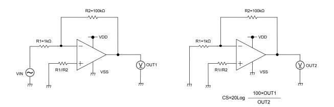
Figure 74. Test circuit 3 (Channel Separation)
