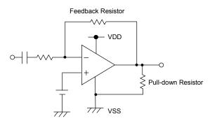
Figure 81. To Suppress the Crosover Distortion
