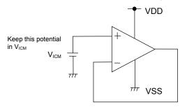
Figure 80. Example of Application Circuit for Unused Op-amp
