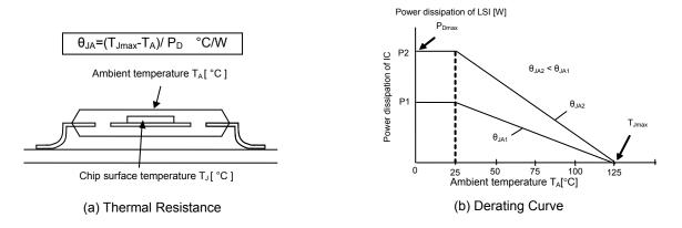
Figure 78. Thermal resistance and Derating Curve
