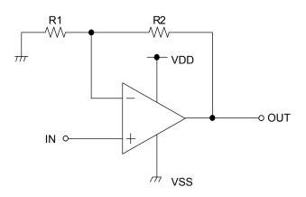
Figure 77. Non-inverting amplifier circuit
