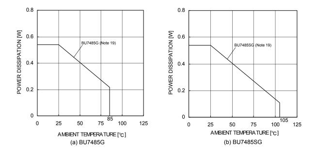
Figure 79. Derating Curve
