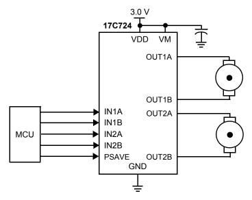
Figure 6. 17C724 Typical Application Diagram
