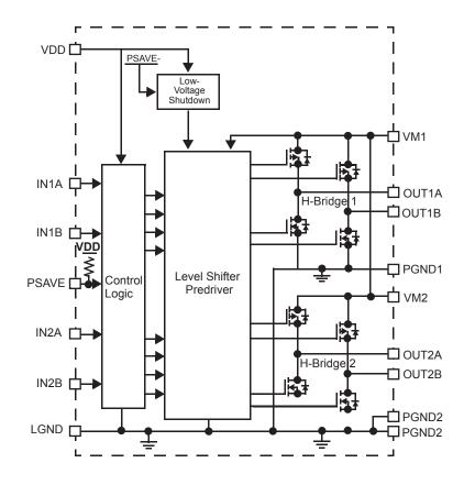
Figure 2. 17C724 Simplified Internal Block Diagram
