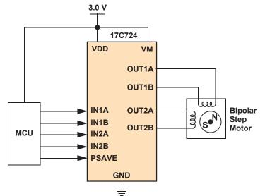
Figure 1. 17C724 Simplified Application Diagram
