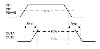
Figure 4.  $t_{PLH}$  and  $t_{PHL}$  Timing
