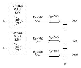
Figure 3. Single versus Dual Transmission Lines
