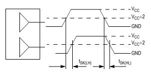
The pin-to-pin skew is defined as the worst case difference in propagation delay between any two similar delay paths within a single device.
