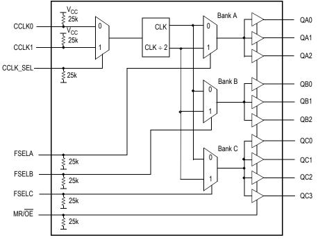
Figure 1. MPC9446 Logic Diagram
