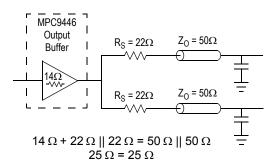
Figure 5. Optimized Dual Line Termination
