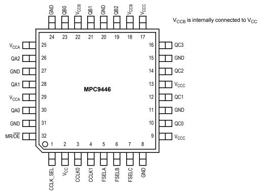
Figure 2. Pinout: 32-Lead Package Pinout (Top View)
