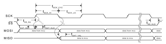
Figure 11. SPI Burst Read Every 9th SCK HI Stretch Timing Diagram
