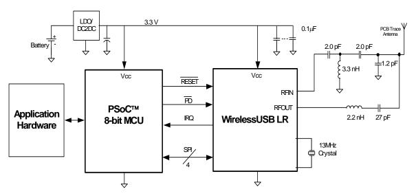
Figure 8. WirelessUSB LR Alarm System
