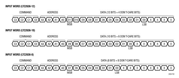
Figure 2. Command and Data Input Format
