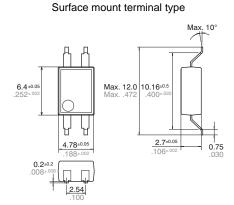
Terminal thickness = 0.20 .008General tolerance:  $\pm 0.1 \pm .004$
