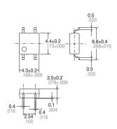
Terminal thickness = 0.15.006General tolerance:  $\pm 0.1 \pm .004$
