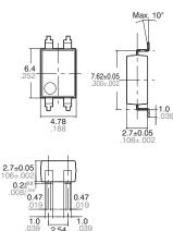
Terminal thickness = 0.2 .008 General tolerance:  $\pm 0.1 \pm .004$
