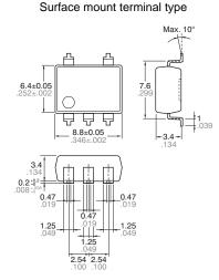
Terminal thickness = 0.25 .010General tolerance:  $\pm 0.1 \pm .004$
