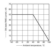
1-(2). ON-state RMS current vs. ambient temperature characteristics
