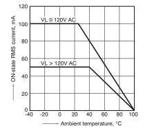
3. Trigger LED current vs. ambient temperature characteristics
