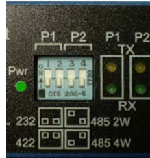
Figure 144: USR602 LED Indicators
