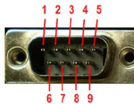
Figure 11: DB-9F Pin Numbering
