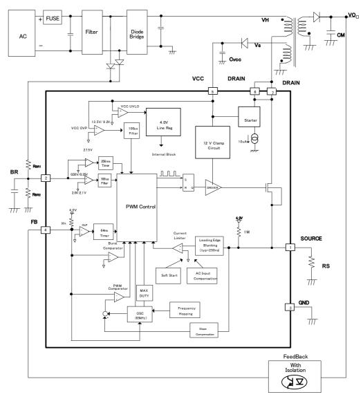
Figure 3. Block Diagram
