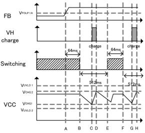
Figure 15. Over load protection (Auto recovery)
