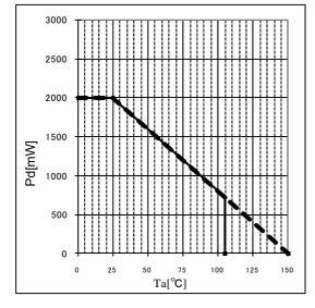
Figure 18. DIP7 Thermal Abatement Characteristics
