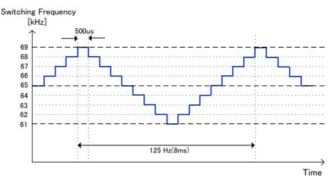
Figure 10. Frequency hopping function
