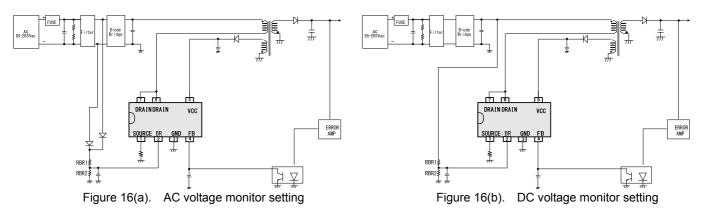
BRUVLO function can protect the breaking of IC when input voltage is low.
