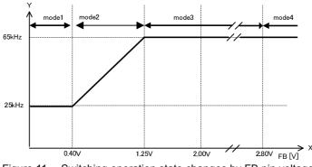
Figure 11. Switching operation state changes by FB pin voltage
