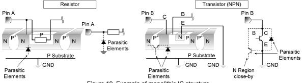
Figure 19. Example of monolithic IC structure
