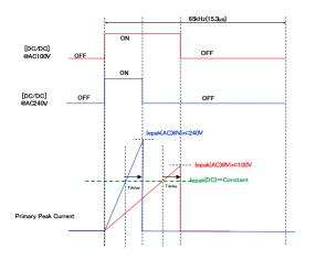
Figure 12. No AC voltage compensation function
