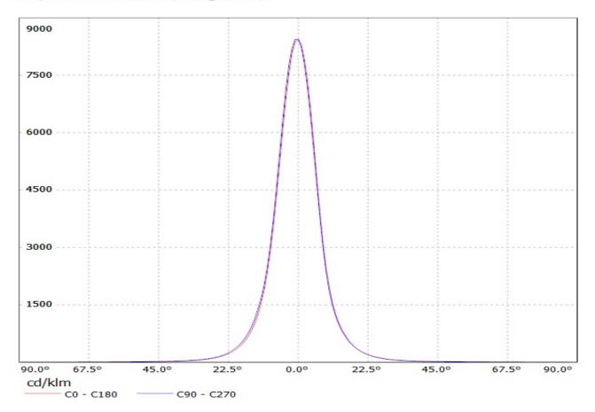
Luminaire: LEDIL OY CP12671\_TINA2-D (XB-D) Efficiency=88% Lamps: 1 x Cree XB-D white (97Im @ 250mA)
