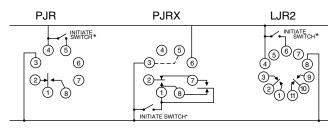
\* INITIATE SWITCH must be isolated from other circuits
