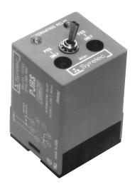
The electronic alternating relay is designed to replace mechanical style devices used in control applications requiring a duplexing or alternating action of the control circuits to operate pumps, compressors, etc. This is achieved by activating a control switch which is common to one side of the input control voltage. The output contact of the relay(s) change state when this switch is opened (on de-energization of the control circuit). When the control
