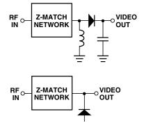
Figure 8. Basic Detector Circuits.
