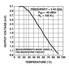
Figure 4. Output Voltage vs. Temperature.
