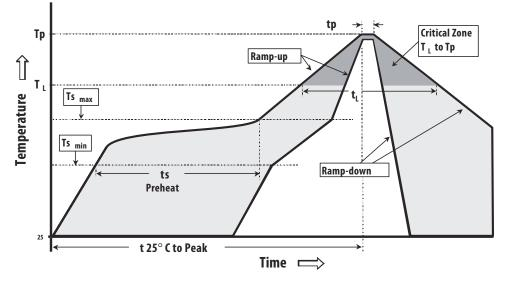
Figure 17. Surface Mount Assembly Profile.
