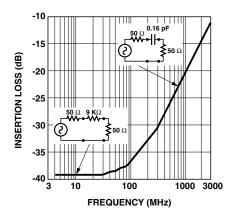
Figure 7. Measuring C<sub>J</sub> and R<sub>V</sub>.
