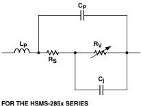
FOR THE HSMS-285x SERI  $C_P = 0.08 \text{ pF}$   $L_P = 2 \text{ nH}$   $C_j = 0.18 \text{ pF}$   $R_S = 25 \Omega$  $R_V = 9 \text{ K}\Omega$
