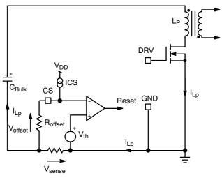
Figure 7. A Simplified Circuit of the Negative Sense Implementation
