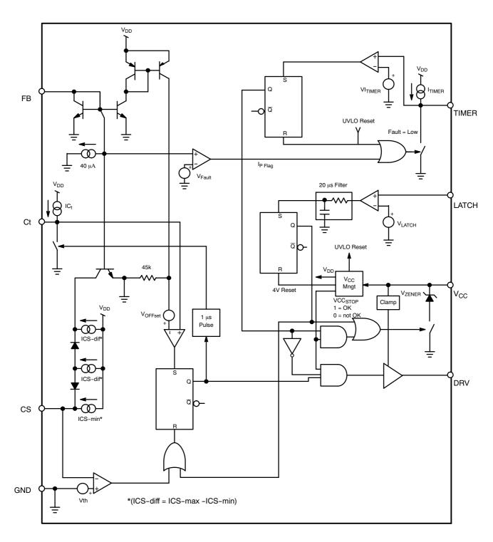
Figure 3. B Version (Auto-recovery Short-Circuit Protection)
