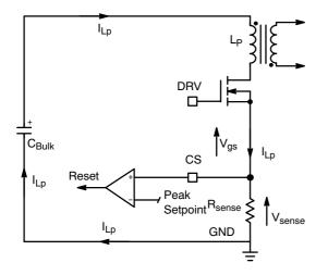
Figure 6. Positive Current-Sense Technique
