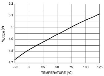
Figure 43. Latch Level Evolution versus Junction Temperature
