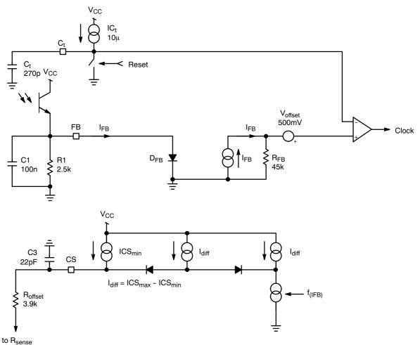
Figure 15. The Feedback Section Inside the NCP1351
