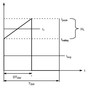
Figure 26. Primary Inductance Current Evolution in CCM
