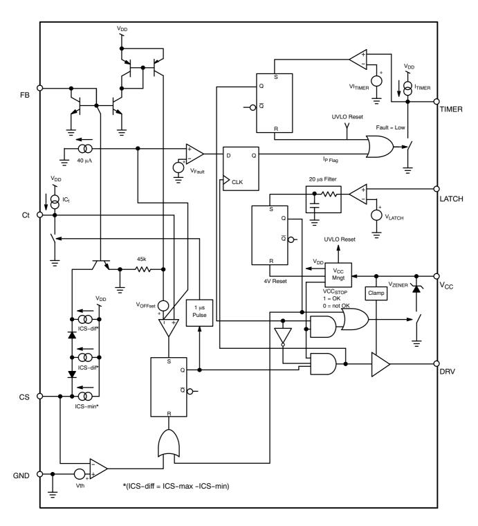
Figure 5. D Version (Auto-recovery Short-Circuit Protection)
