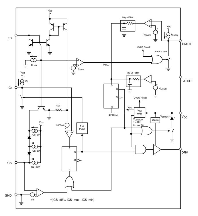
Figure 2. A Version (Latched Short-Circuit Protection)
