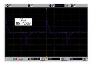
Figure 31. Transient Step, Low Line
