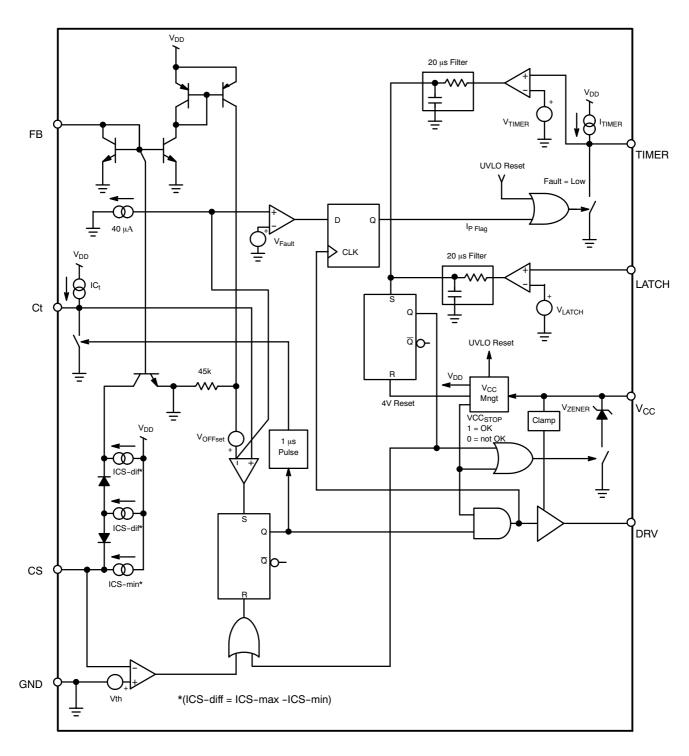
Figure 4. C Version (Latched Short-Circuit Protection)
