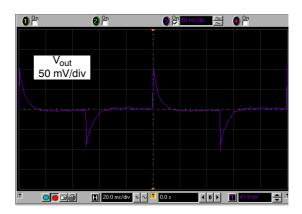
Figure 32. Transient Step, High Line
