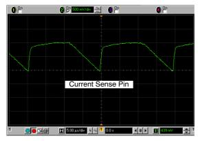
Figure 8. The Voltage on the Current Sense Pin
