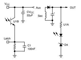
Figure 25. You can either directly observe the V<sub>CC</sub> level or add a small RC filter to reduce the leakage inductance contribution. The best is to directly sense the output voltage and reacts if it runs away, as offered on the right side.
