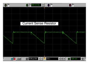
Figure 9. The Voltage Across the Sense Resistor
