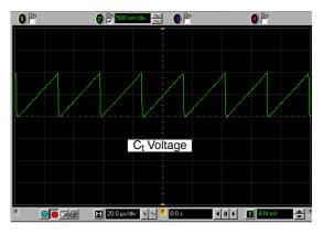
Figure 12. Ct Voltage Swing at a Moderate Loading
