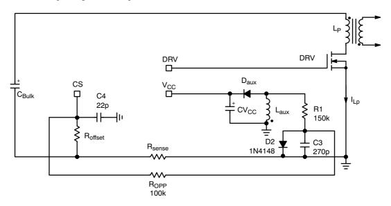
Figure 14. The OPP is Relatively Easy to Implement and It Does not Waste Power
