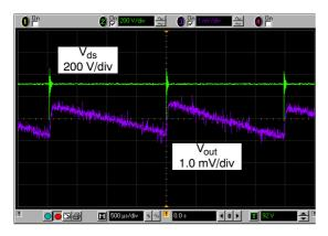
Figure 29. No-Load Output Ripple (V<sub>in</sub> = 230 Vac)
