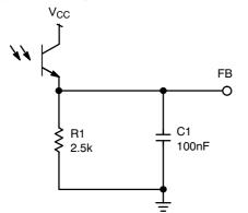
Figure 17. The Recommended Feedback Arrangement Around the FB Pin
