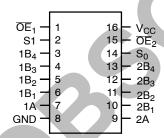
Figure 1. 16-Lead Pinout
