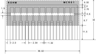
The shaded area shows the solder resist treatment. NOTE) \*1
