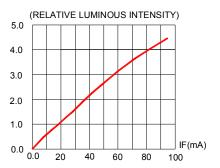
$\begin{aligned} & \textbf{FIG.2 RELATIVE LUMINOUS INTENSITY VS.} \\ & & \textbf{FORWARD CURRENT} \end{aligned}$
