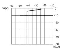
FIG.3 REVERSE CURRENT VS. REVERSE VOLTAGE.
