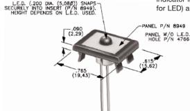
PANEL INSERT BLANK PANEL INSERT WITH HOLE FOR LED WITHOUT HOLE FOR LED
